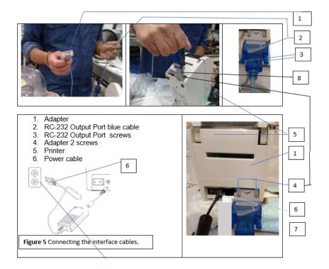
4. Connect the power cable connector of cable (6) coming from the printer to the electrical power source on the wall.
