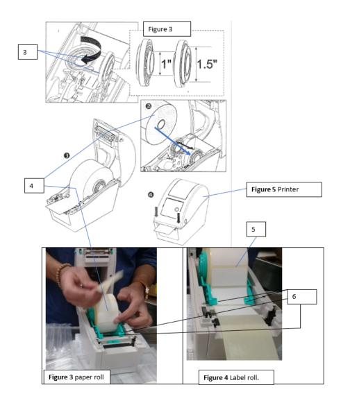
6. Push the printer cover down (fig 5) until you can hear a click indicating that the cover is connected to the printer bottom.
