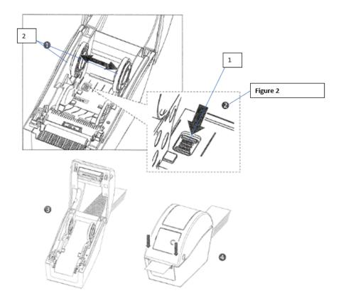
5. Insert the paper under the two paper guides (item 6) in figure 3 for the paper roll, pull the paper to extend it beyond the printer. Do the same for the label roll (item 6) figure 4.
