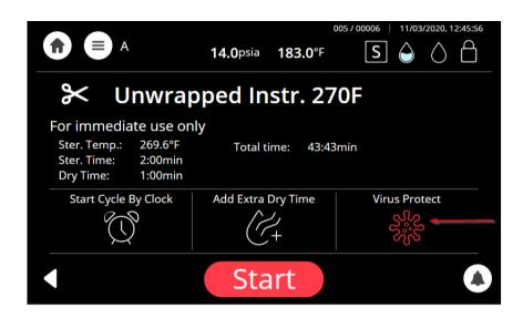
2. Raise the temperature to 230°F (110°C) and wait for a period of 10 minutes, for the Virus Protect process to complete and if, for example, the Unwrapped Instr. sterilization program is selected, the screen below is displayed if the virus protect is successfully completed.
