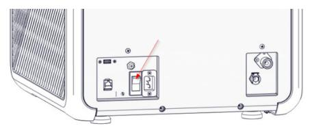
Turn on the ON/OFF switch mounted under the cover on the front of the autoclave (see below)
