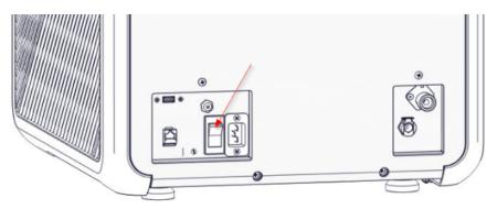
3. Turn on the ON/ OFF Switch mounted on the bottom left side of the front panel (see the front view).
